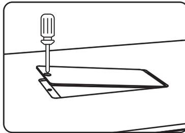
2. Pull open the fastening clip to install the SSD, secure the SSD by pressing the clip, then restore the screws and cover.
