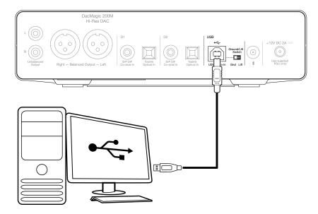
The DacMagic 200M only supports USB audio playback using USB Class 2.0 Audio. For this it is required that the DacMagic 200M is connected to a USB 2.0 port using a suitable USB cable, and we would recommend any USB certified high-speed USB 2.0 'A-B' cable.
